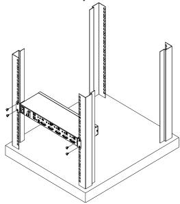
**Note:** These screws are not provided. We recommend that you use M5 x 12 Phillips Type I cross, recessed type screws.
